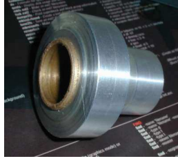
Figure 3: Pilot bush adapter bush, the bronze bush has been fitted.
